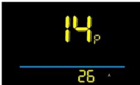
Figure 3-14 Controller Current limit setting interface
