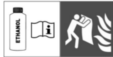
Adhere to instructions about fuel. ISO 7010-F016, Fire blanket
