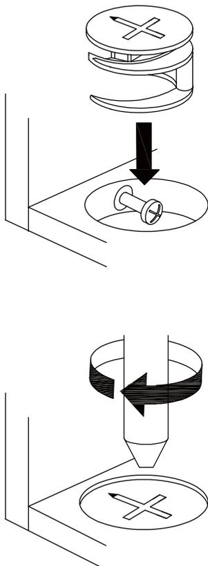
**EN\_Quickfit head** should be in the centre of the cam lock when the two panels are joined.
