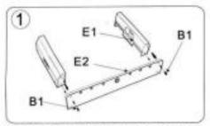
Assemble two short boards and one long board, then connect by screws.
