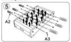
Insert six handles and six cover into the bars, make sure that all the handles are tightened.
