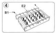
Insert the last long board right to the position of the bars ,then screw it in.
