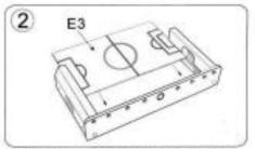
Insert the bottom board into the assembled boards of 1step.
